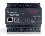
The communication between the Solar-Log<sup>™</sup> Smart Relay Station and the Solar-Log<sup>™</sup> takes places via a network interface RJ45 (TCP/IP).
