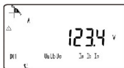
Voltage on A phase
