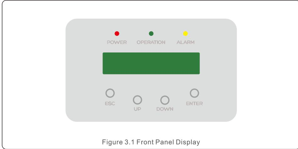
Figure 3.1 Front Panel Display
